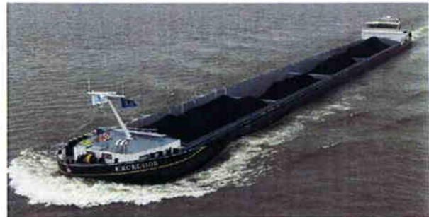
Combi International's Excelsior, a 135-meter/443-foot dry cargo ship powered by twin 1,260-horsepower Mitsubishi S12R-C2MPTK engines, was built in 2008.
